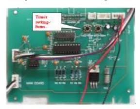
Timer Control Board takes pulse signal from the AC5 Coin Accepter and converts the pulse to time on timer (minutes per pulse).
