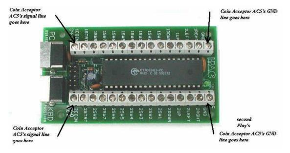
6.2 Connect hacked keyboard, you can connect the signal line and GND line into Key 1 whichever MAME coin key connect to.
